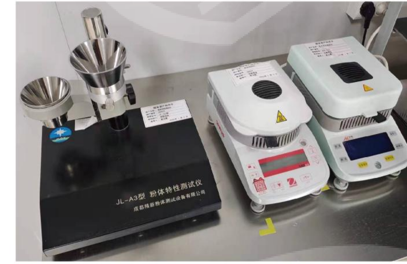
粉体特性和含水率测试设备 Powder performance and moisture content testing equipment
